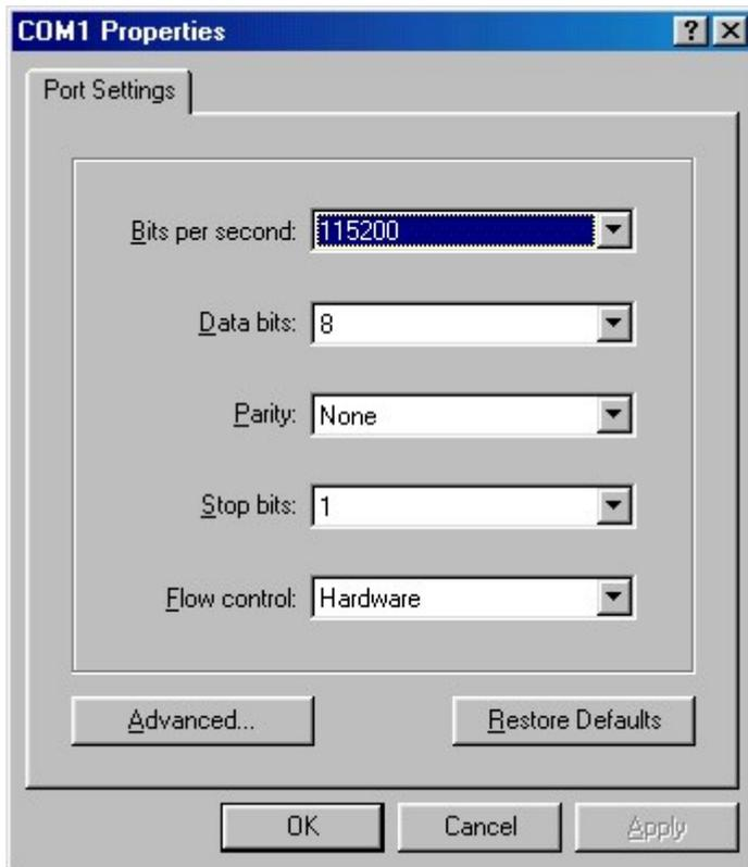
Configure the serial port as shown in the screen on the left.
